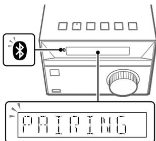
"PAIRING" flashes on the display [10] and the
