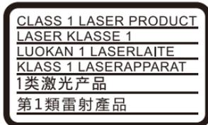
This appliance is classified as a CLASS 1 LASER product. The CLASS 1 LASER PRODUCT MARKING is located on the rear exterior.
