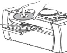
Press **▲** on the unit again to close the disc tray. Do not forcibly push the disc tray to close it as this may cause a malfunction.
