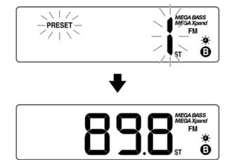
The display shows the frequency for about 10 seconds, and then returns to the current time.
