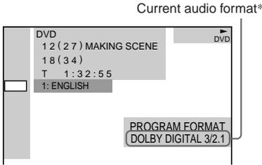
\*“PCM,” “MPEG,” “DTS,” or “DOLBY DIGITAL” is displayed. For “DOLBY DIGITAL,” the channels in the playing track are displayed numerically as follows:
