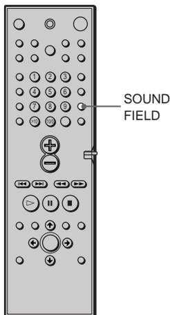
Press **SOUND FIELD**  $-/+$  on the system or **SOUND FIELD** on the remote repeatedly until “2CH STEREO” appears on the front panel display.
