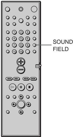
Press **SOUND FIELD**  $-/+$  on the system or **SOUND FIELD** on the remote repeatedly until **"AUTO DECO.(AUTO DECODING)"** appears on the front panel display.
