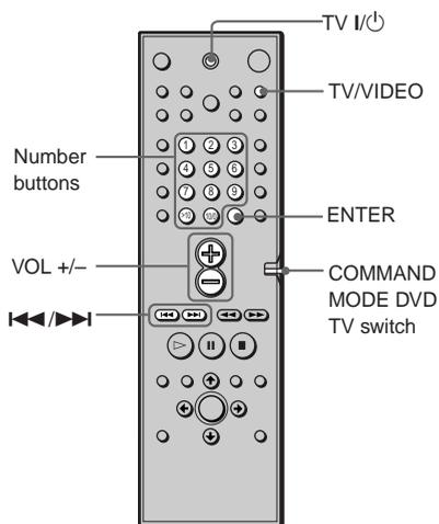
Press and hold TV I/O while entering your TV's manufacturer's code (see the table) using the number buttons and press ENTER. Then release TV I/O.
