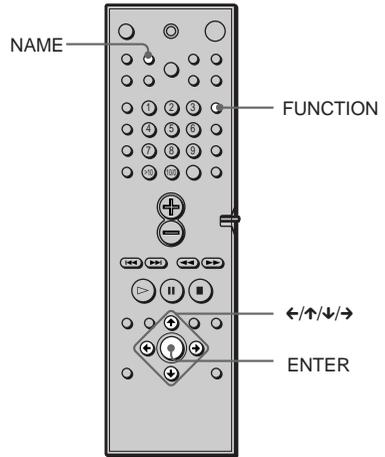
**1** Press **FUNCTION** repeatedly until **TUNER** appears on the front panel display.
