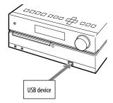
When USB cable connection is necessary, connect the USB cable supplied with the USB device to be connected.
