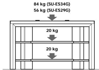
Do not place any equipment which exceeds the maximum weight for each divider as indicated in the illustration. Otherwise, the divider may break.
