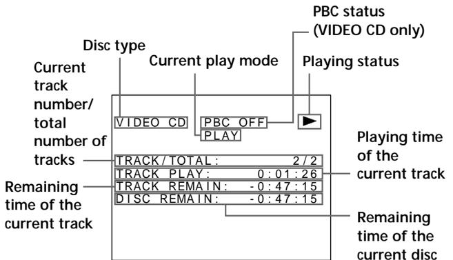
During Shuffle Play or Program Play, the remaining time of the disc is not displayed.
