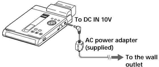
**3** Disconnect the AC power adapter from the player and pull out from the wall outlet after charging.
