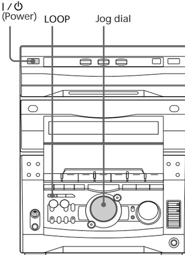
➔ Press and hold LOOP during playback at the point you want to start the Loop function, and release to resume normal play.
