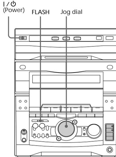
➔ Press and hold FLASH during playback at the point you want to start the Flash function, and release to resume normal play.
