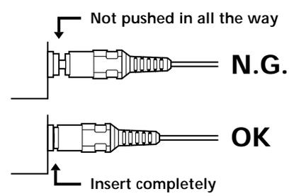
**Connecting the power cord to an AC outlet**
