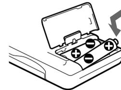
② Install two size AA (LR6) alkaline batteries (not supplied), and close the lid.
