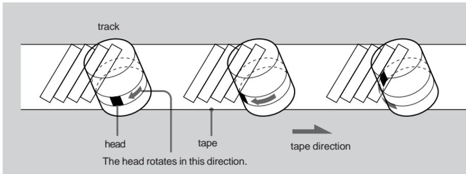
On the other hand, with the NT (Non-Tracking) format, a rotary head is not required to precisely trace the recorded track during playback. Therefore, the number of mechanical parts has been reduced. And this makes the compact size of the recorder possible.
