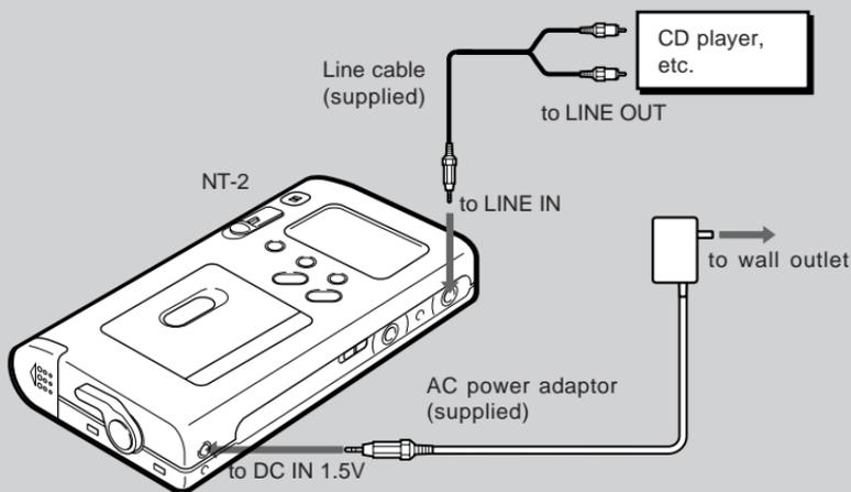
The recorder is operable on AC power using the AC power adaptor (supplied).
