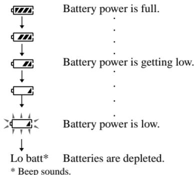
When the batteries are depleted, replace both batteries with new ones.
