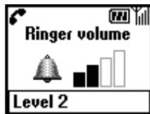
During a call, you can adjust the speaker volume by rotating the Jog Dial. Rotate up to increase the volume and down to decrease the volume.
