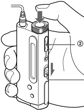
② Press the VOLUME +/- button up or down to adjust the volume.
