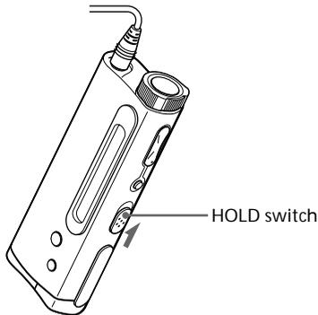
Slide the HOLD switch in the direction of the arrow.
