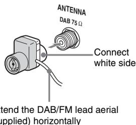
Connect a DAB external aerial (not supplied) to the DAB terminal on the back of this unit.
