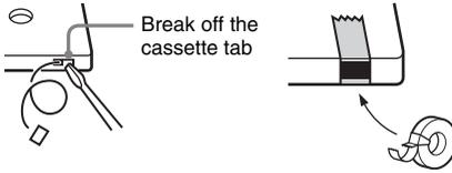
If you later want to reuse the tape for recording, cover the broken tab with adhesive tape.
